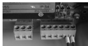
Fig. 15: Connecting an external alarm
