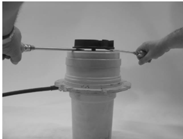
Fig. 26: Lifting off the impeller
