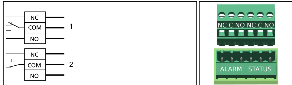
Fig. 10: Wiring diagram for the general fault message
