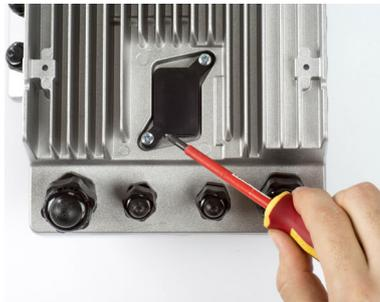
Fig. 25: Inserting and fastening cover
