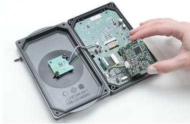
Fig. 49: Installing the Bluetooth module
