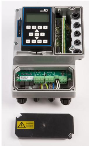
**Fig. 14:** Removing the protective cover
