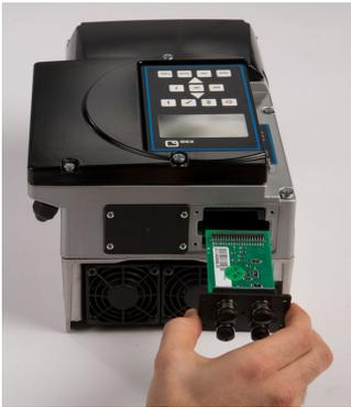
Fig. 42: Inserting the field bus module
