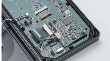
Fig. 50: Securing the Bluetooth module
