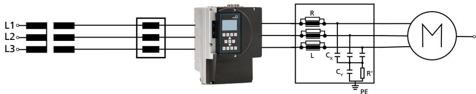
Fig. 31: Installing line choke and output filters
