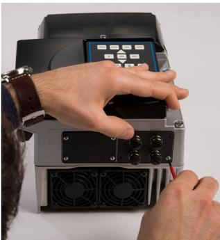
**Fig. 36:** Securing the M12 module
