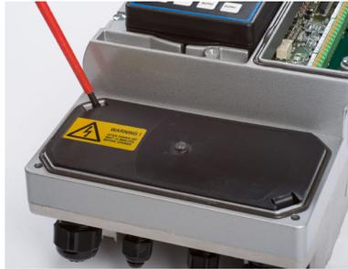
**Fig. 13:** Prying open the protective cover
