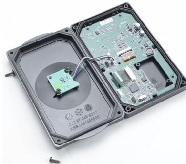
**Fig. 48:** Open graphical control panel
