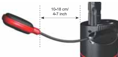
Fig. 4 Minimum free cable length for float switch
