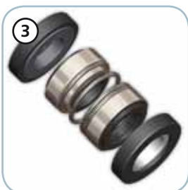
Mechanical seal Three mechanical seals; double seal (SiC-Al) in oil sump with food-grade oil lubrication, one V-ring in direct contact with the liquid.
