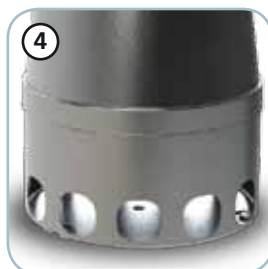
Strainer Chrome-nickel steel AISI 304 Max free passage 40 mm.
